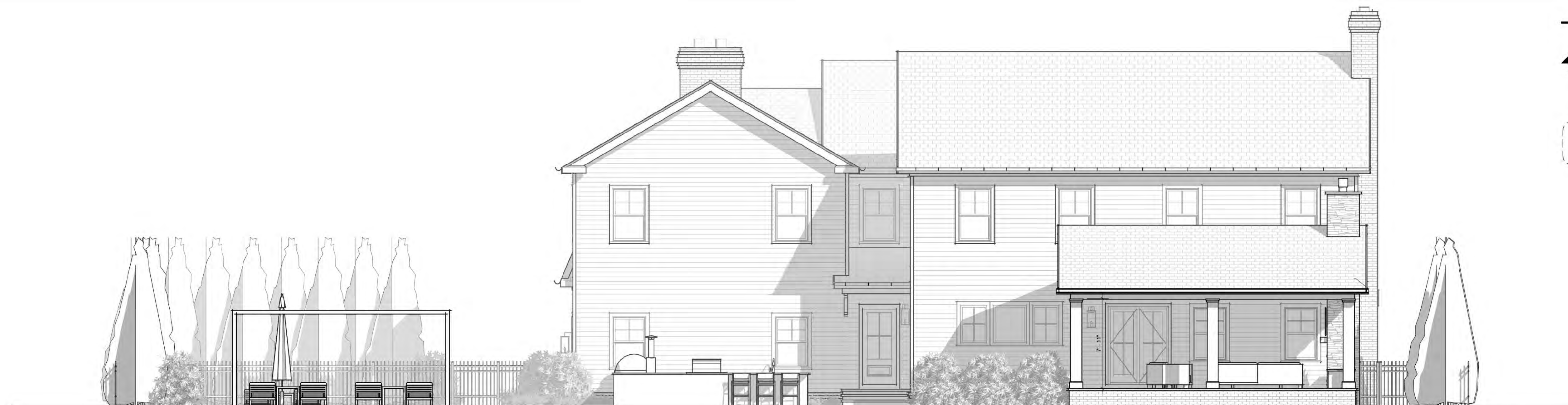
Proposed Rear Patio Elevation 3/16" = 1'-0"
