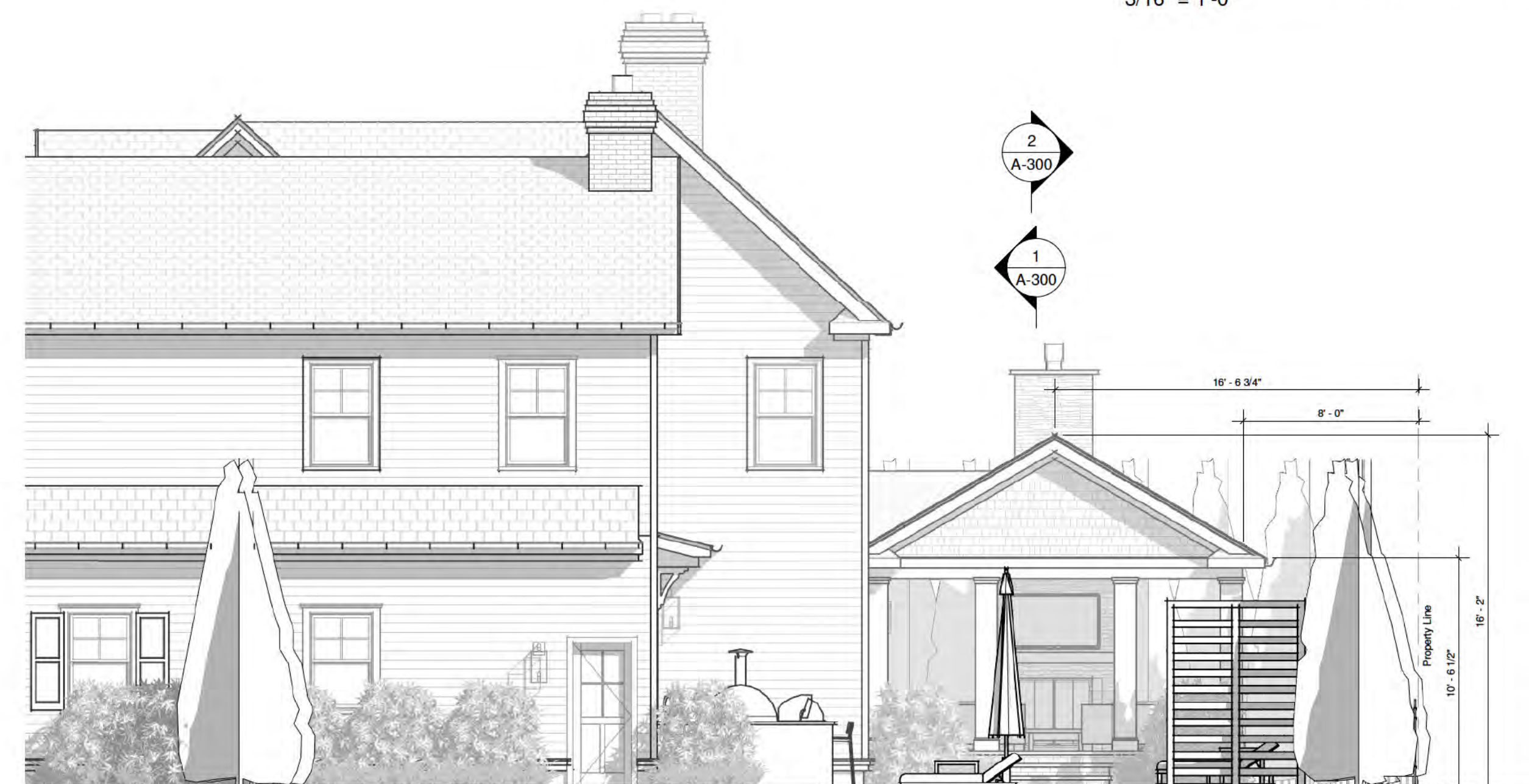
Proposed Right Side Patio Elevation 3/16" = 1'-0"
