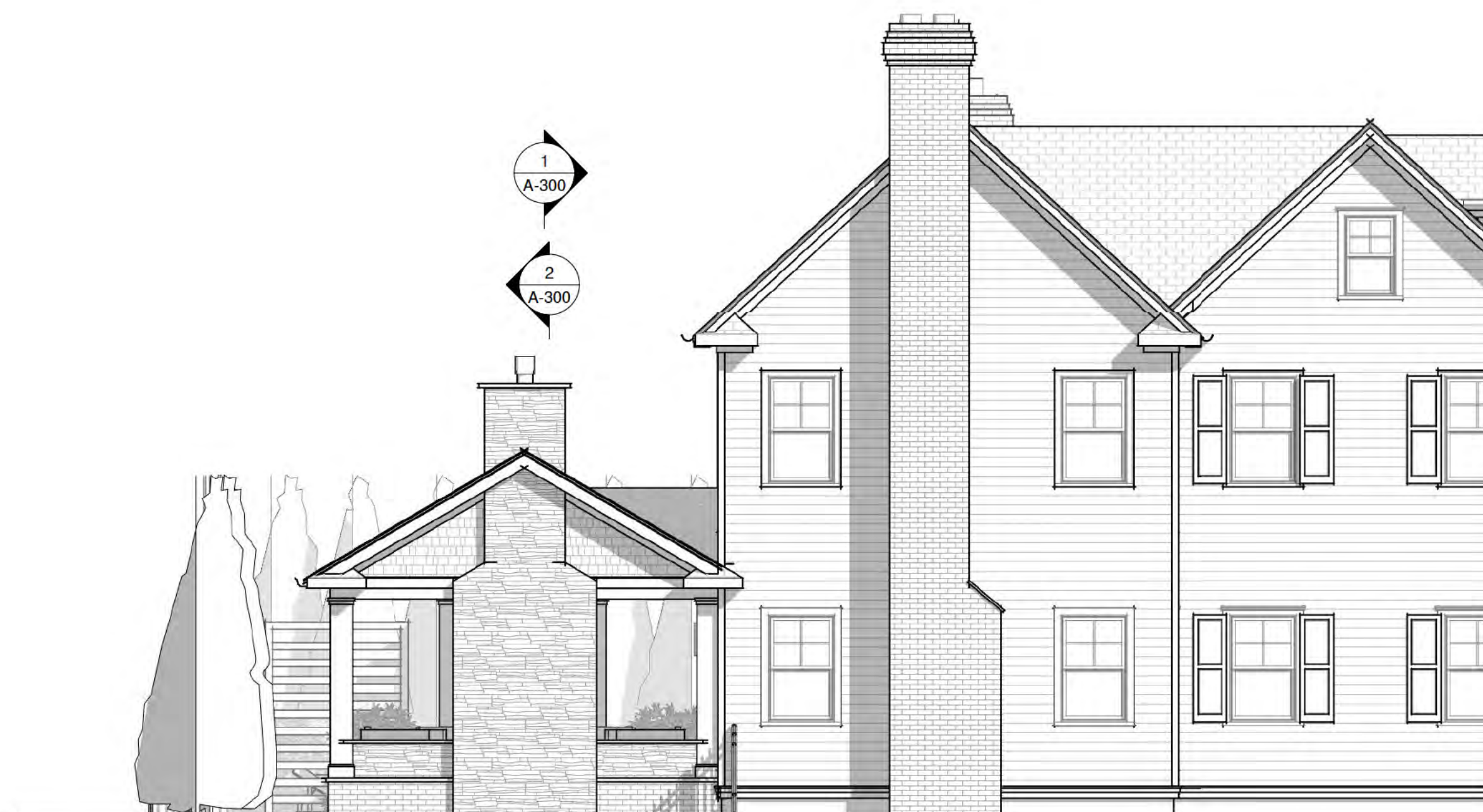
Proposed Left Side Patio Elevation 3/16" = 1'-0"
