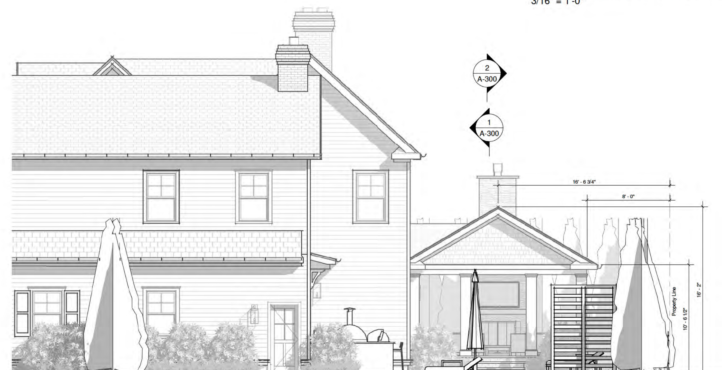
Proposed Right Side Patio Elevation 3/16" = 1'-0"
