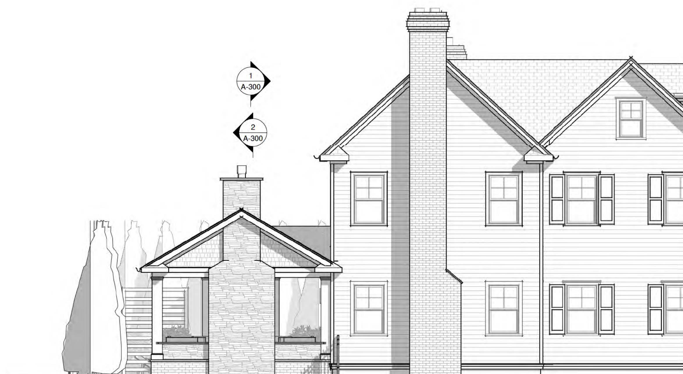
Proposed Left Side Patio Elevation 3/16" = 1'-0"
