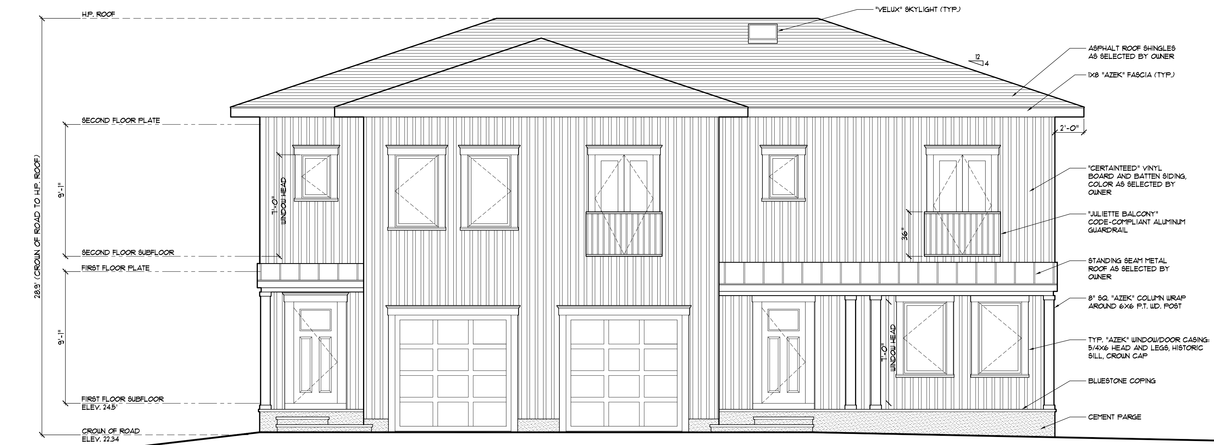
FRONT (SOUTH) ELEVATION 1/4" = 1'-0"
